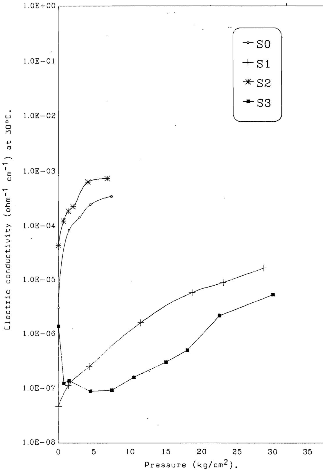
**Figure (10) Dependence of the electrical conductivity on the hydrostatic pressure (at 30 C).**
