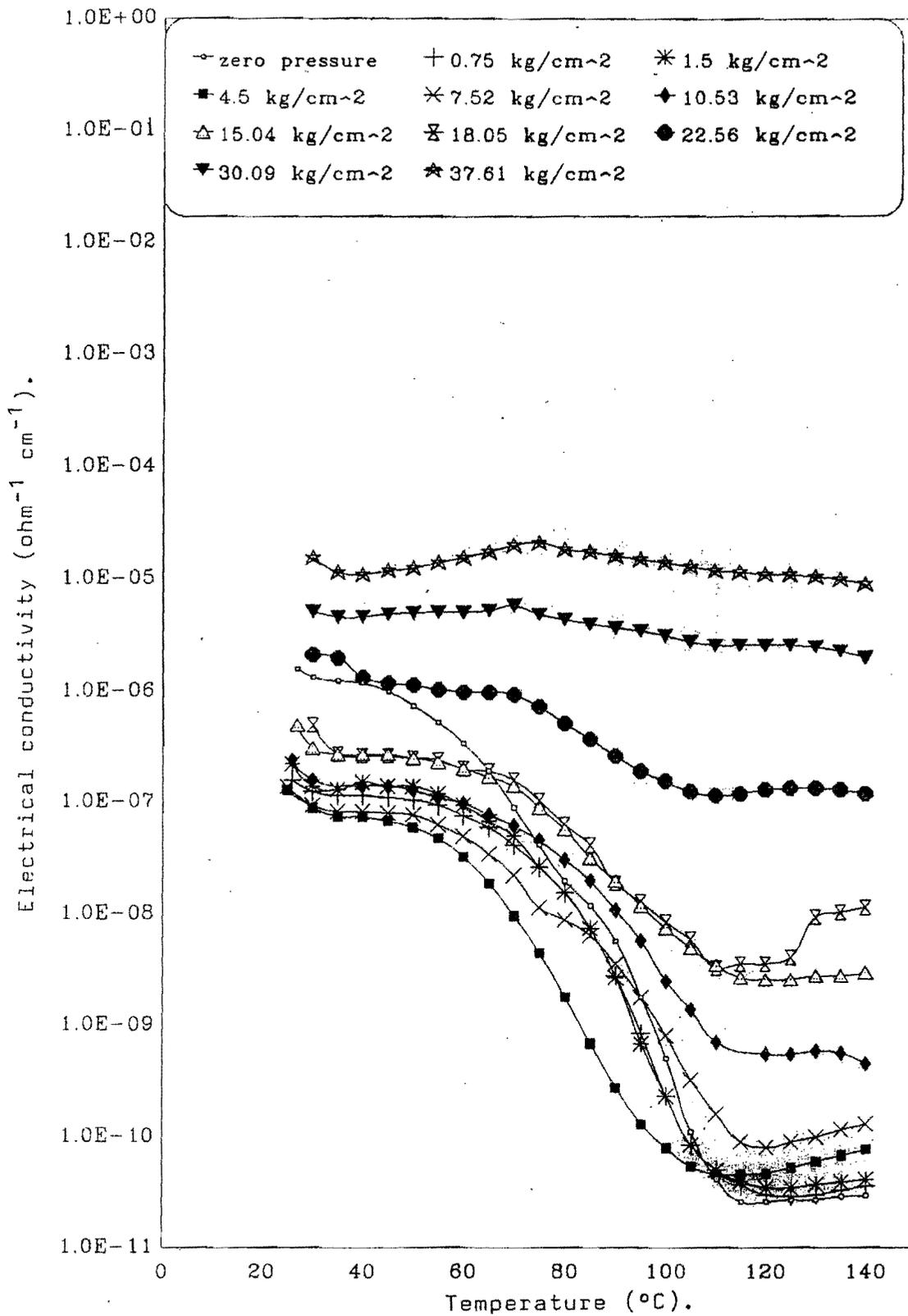
Figure (9) Temperature dependence of electrical conductivity for S3.
