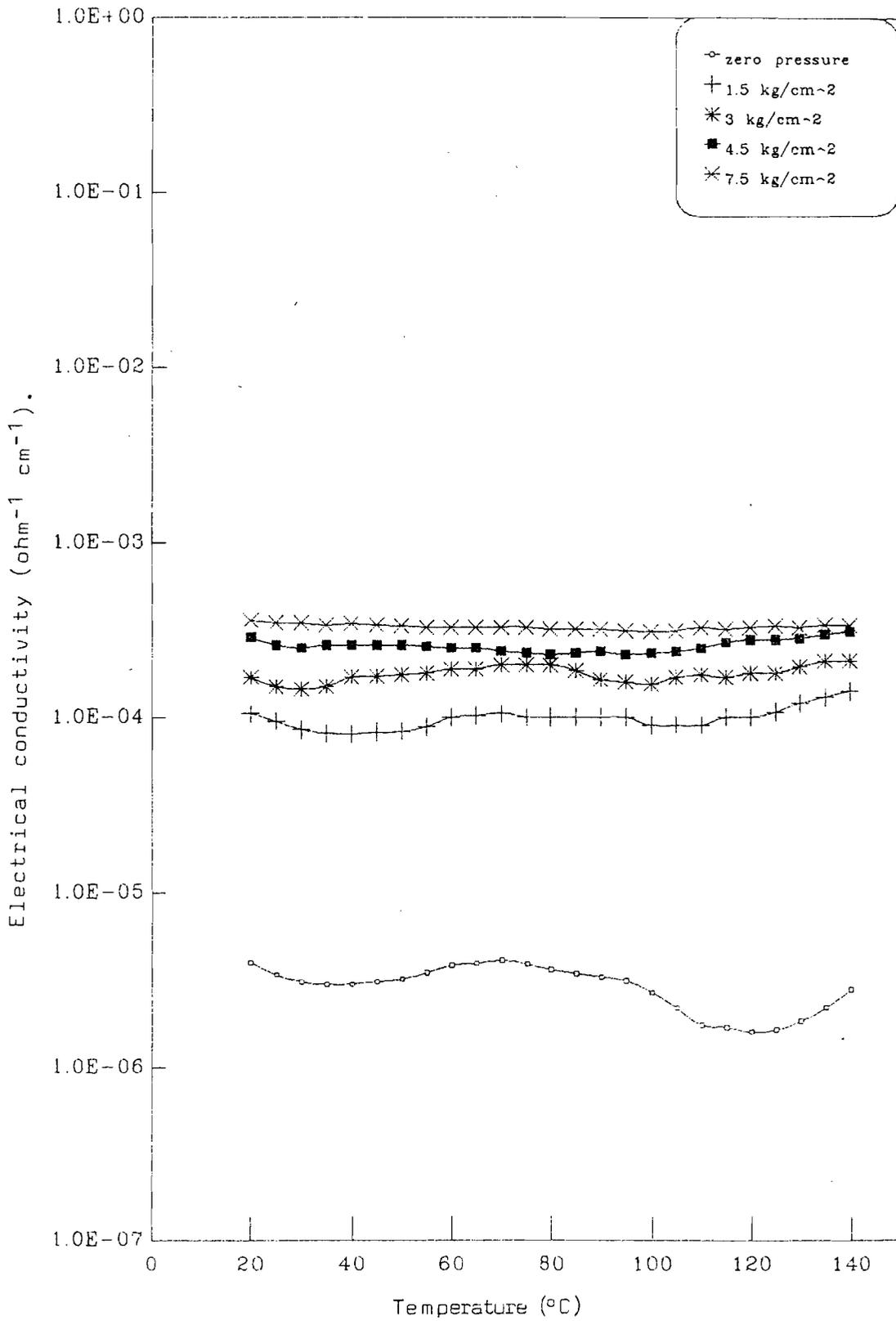
Figure (6) Temperature dependence of electrical conductivity for S0.
