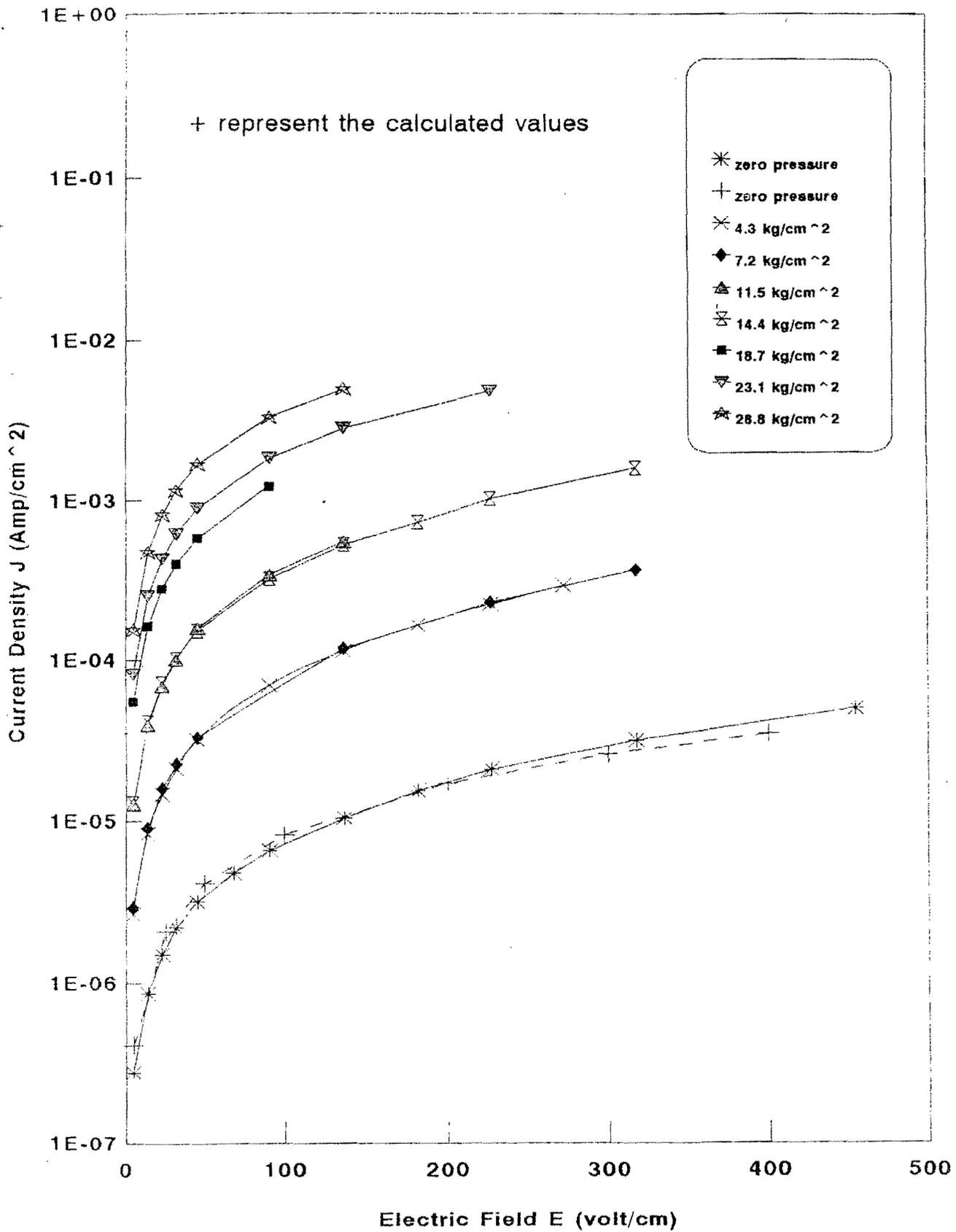
Figure (3) Dependence of log J vs. E curves on hydrostatic pressure for S1.
