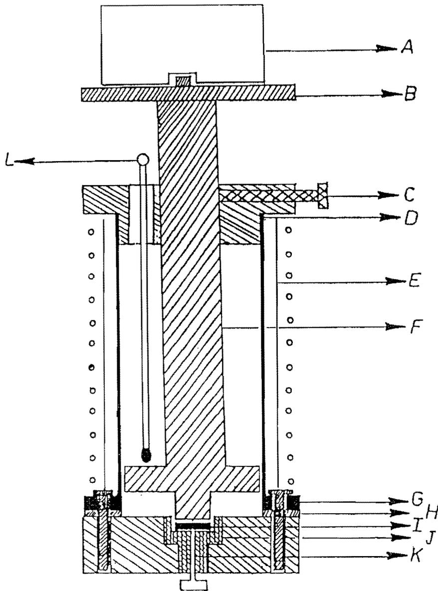
Figure (1) : Schematic diagram for the device used to carry out the electrical conductivity measurements, for pre-compressed samples .
