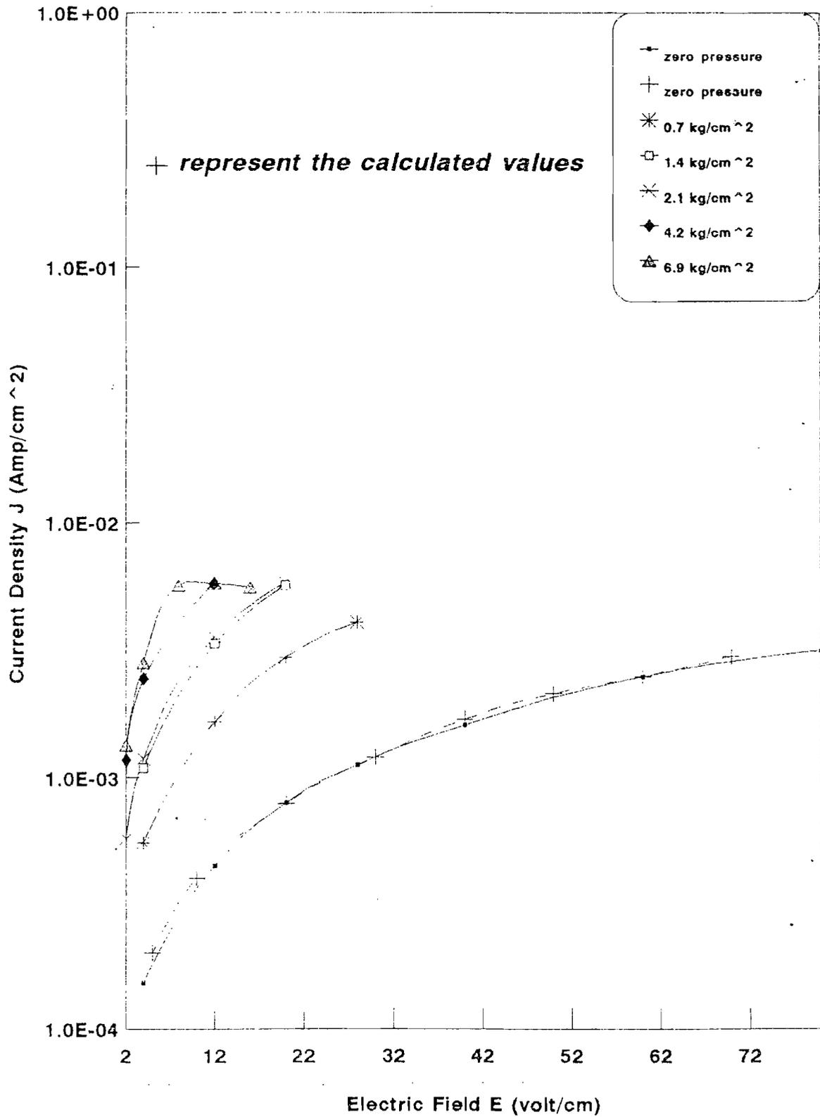
**Figure (4) Dependence of log J vs. E curves on hydrostatic pressure for S2.**
