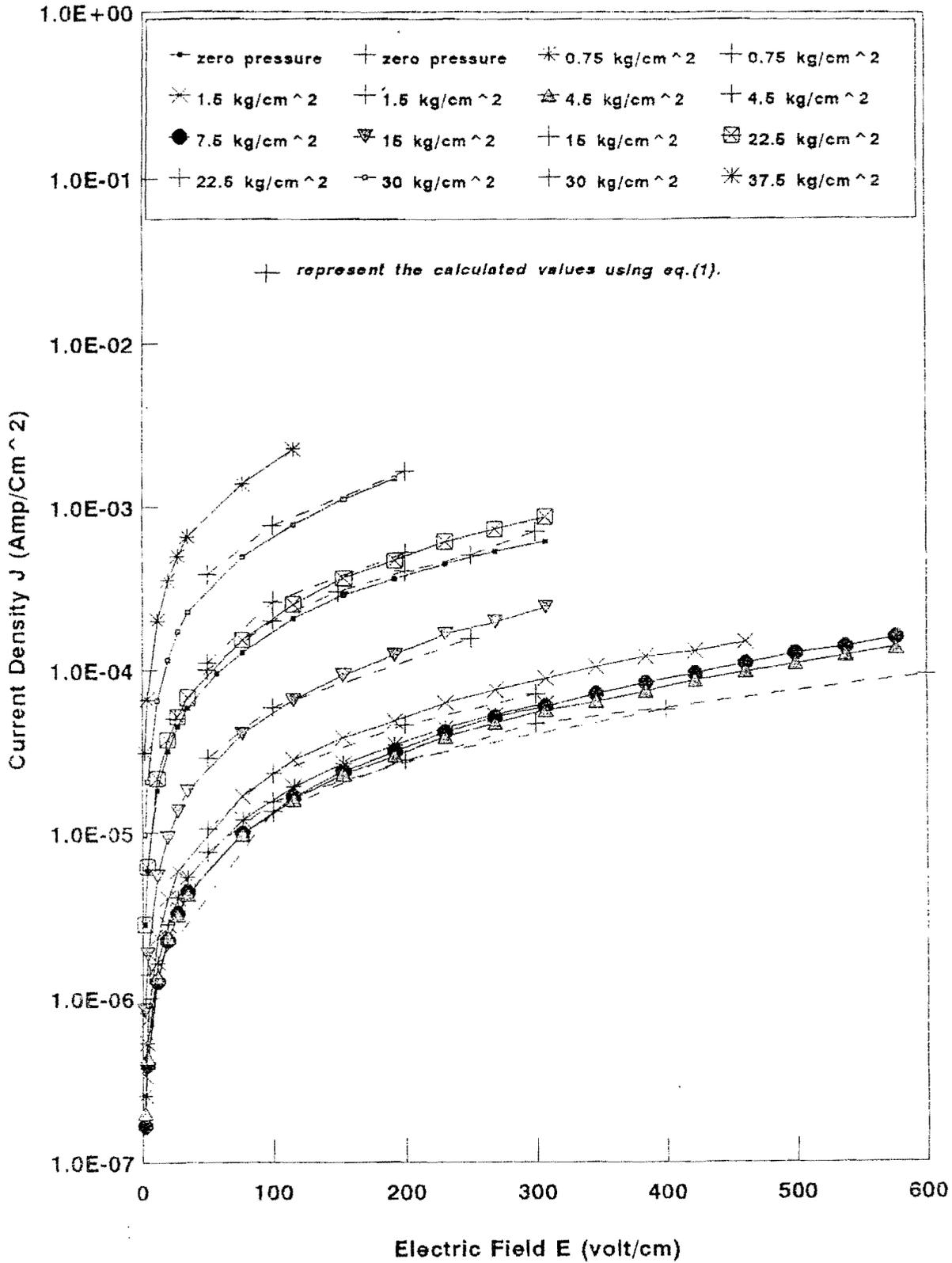
Figure (5) Dependence of log J vs. E curves on hydrostatic pressure for S3.
