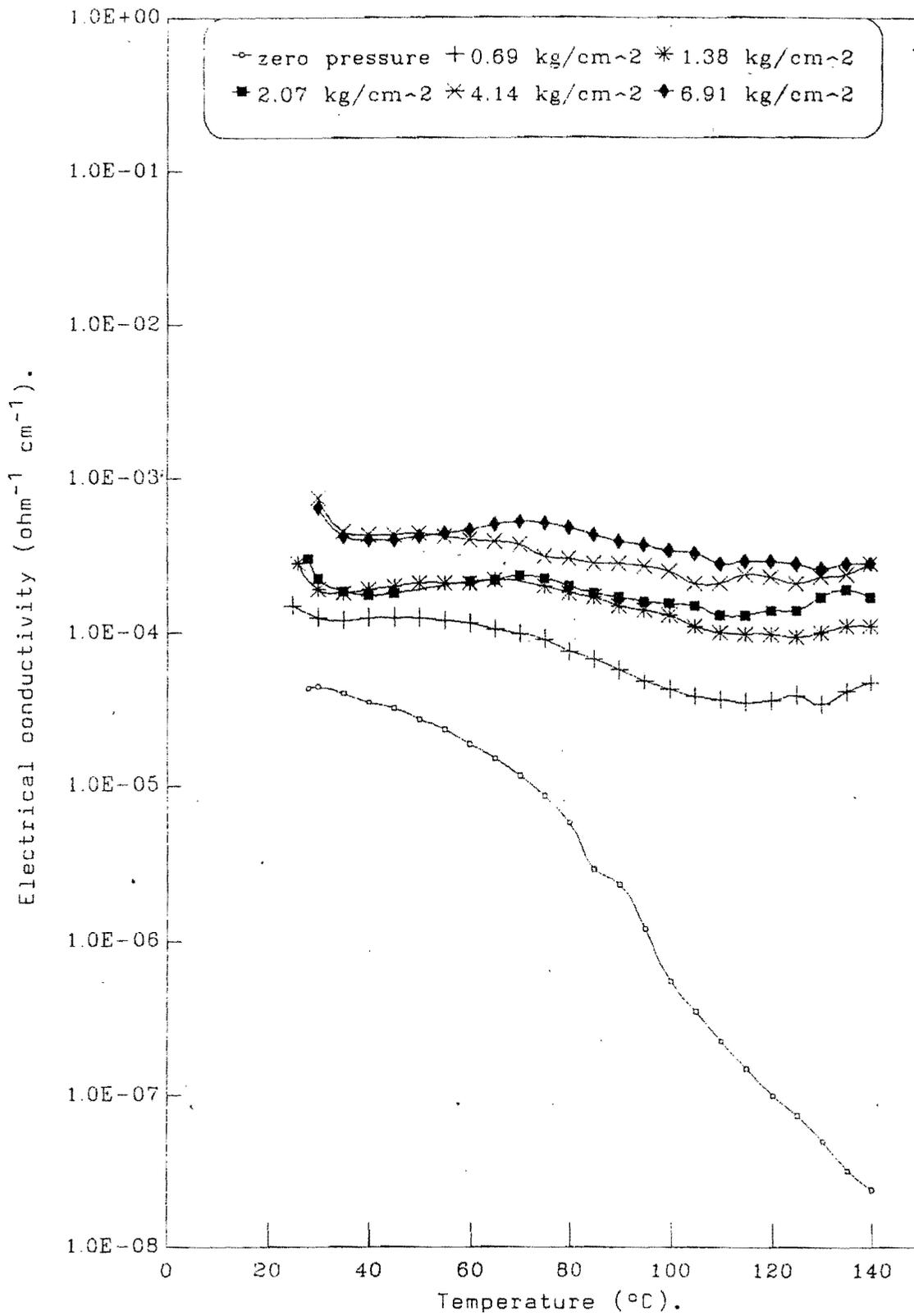
Figure (8) Temperature dependence of electrical conductivity for S2.
