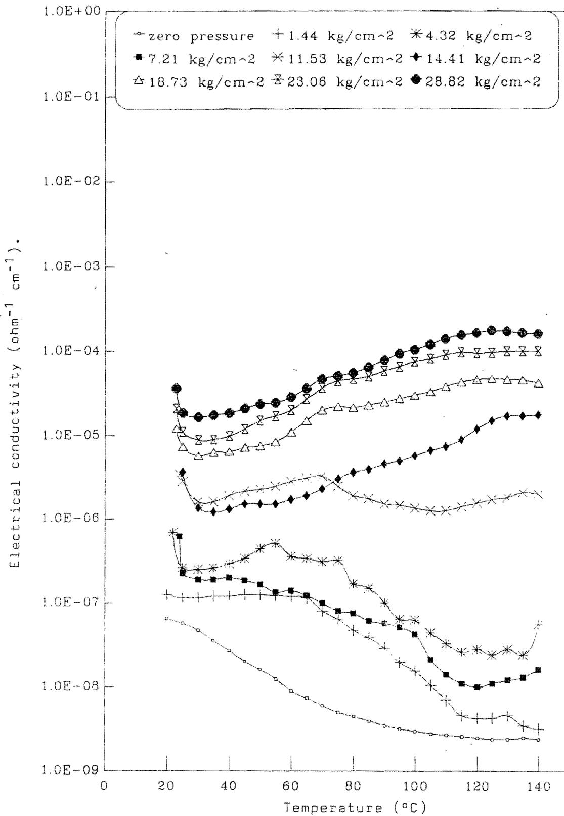
Figure (7) Temperature dependence of electrical conductivity for S1.
