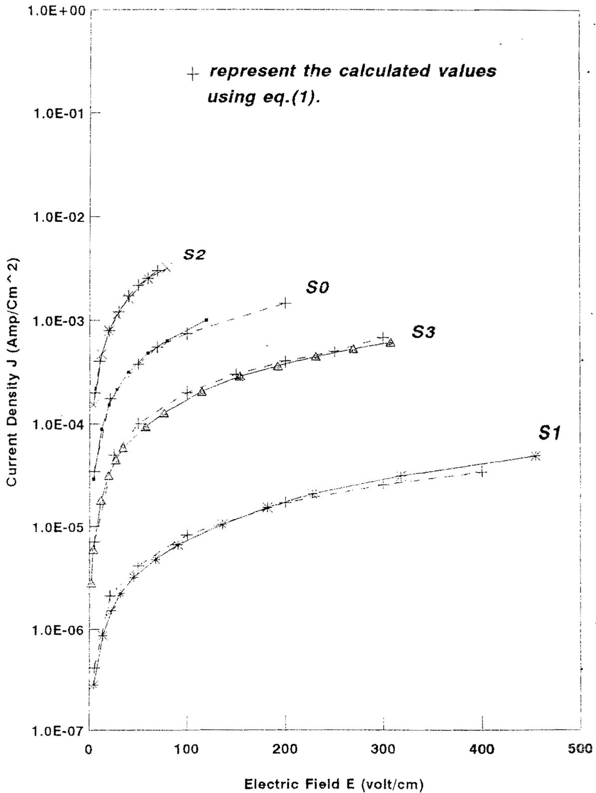
Figure (2) Current density J vs. electric field E curves for different composites at zero pressure.
