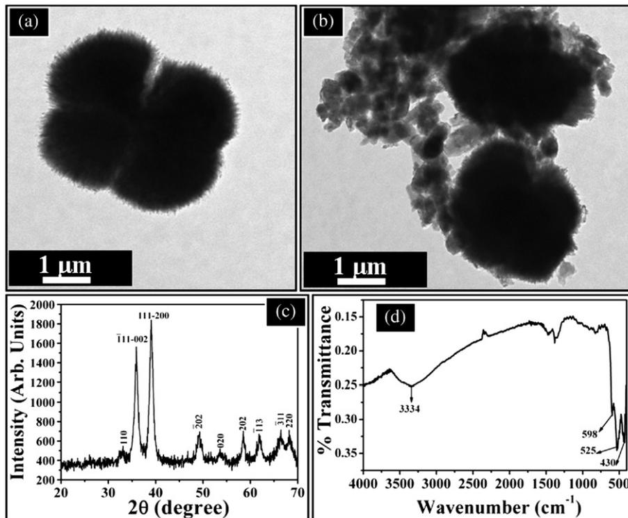
Fig. 3. (a) and (b) Typical TEM images; (c) X-ray diffraction (XRD) pattern and (d) FTIR spectrum of the as-grown urchin-like CuO structures grown by simple solution process.
