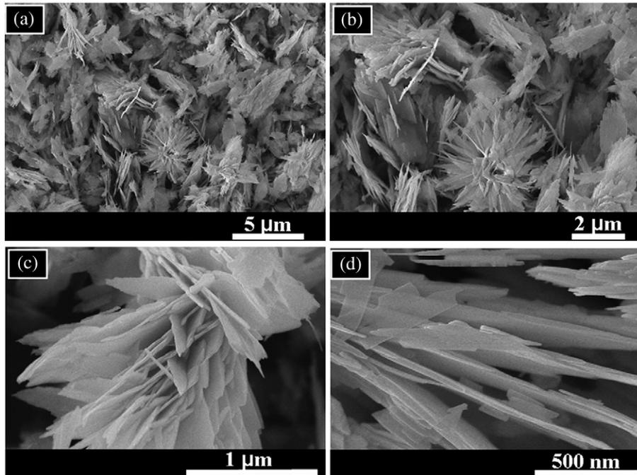
Fig. 2. (a) and (b) Low and (c) and (d) high-magnification typical FESEM images of flower-like composed of thin nanosheets and irregularly arranged sheet-like structures grown in the reactant solution.
