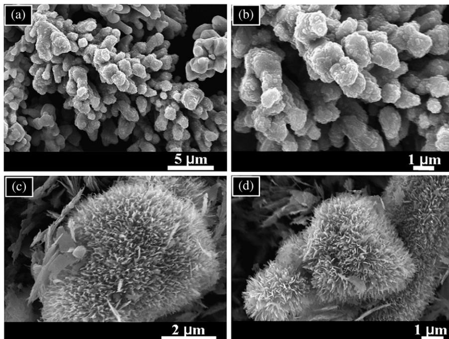
Fig. 1. (a) Low and (b) high-magnification typical FESEM images of copper powder before the experiment and (c) low and (d) high-resolution FESEM images of as-grown urchin-like CuO structures grown onto the copper powder by simple solution process.
